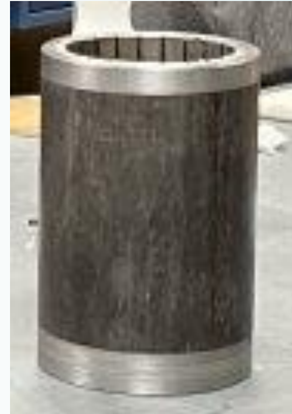
Ring gear with machined ends
