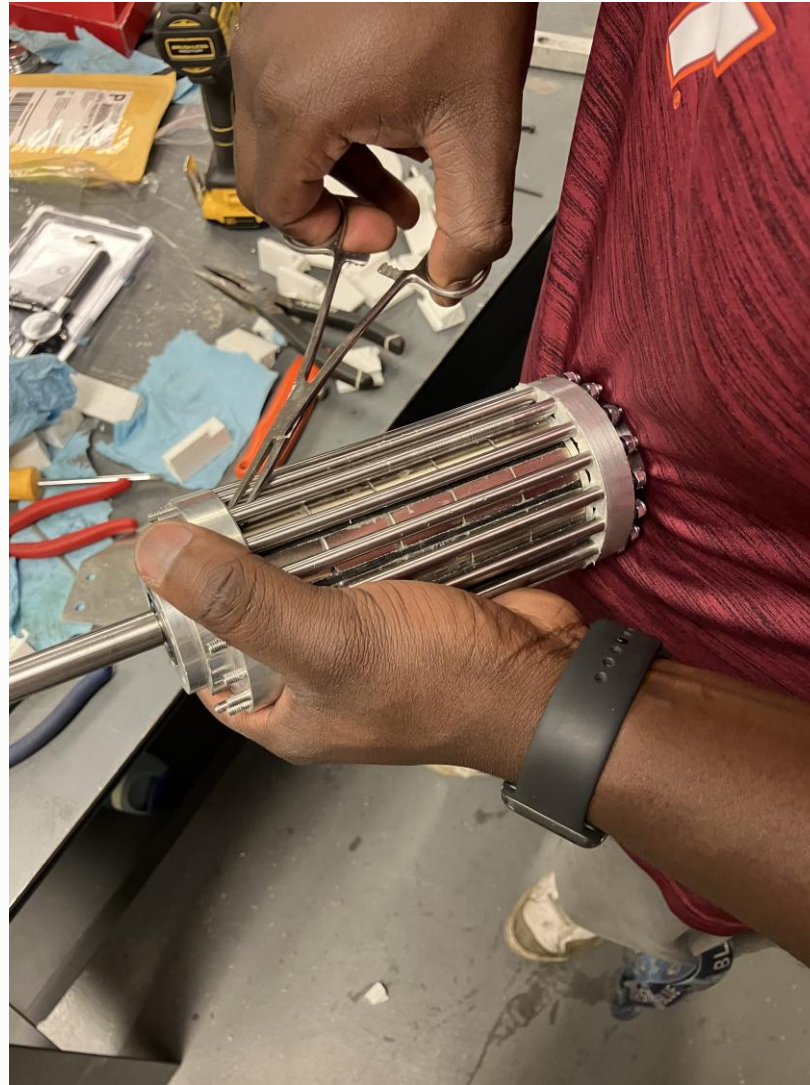
Putting the Modulator around the Sun Gear
