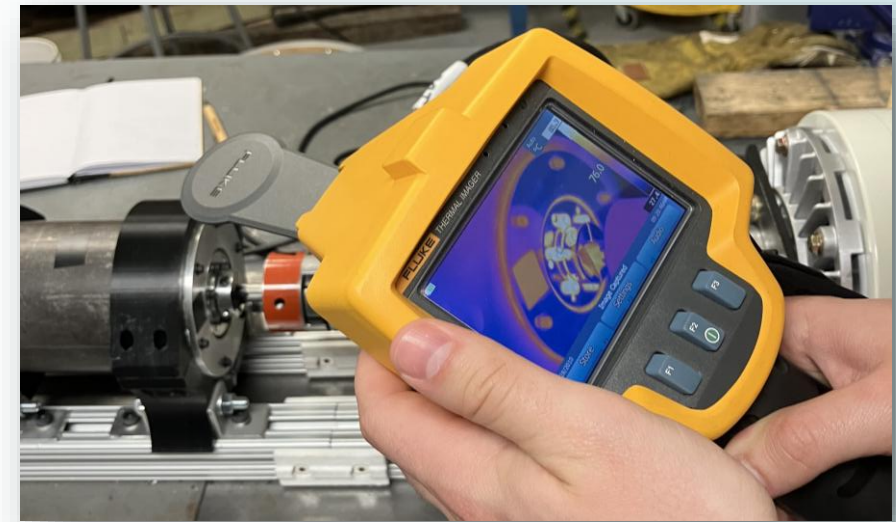
FLUKE Thermal Camera in use (max 76° C)
